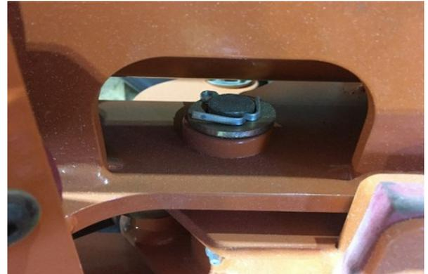
Another area that requires your attention are the cotter pins that retain the (6) Linkage Pins. The cotter pins can rot out in colder climates where salt is used on the roads. Once the cotter pin fails the linkage pin can fall out. Inspect and replace the cotter pins as needed.
