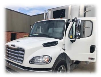
Air brakes and low-profile tires provide better driving characteristics along with lower height (under 12' in NON-CDL) improving fuel economy and allowing access to some height restriction areas. These new "PLUS" chassis will hopefully be coming in beginning of the new year and we believe this will be a winning combination moving forward. Give us a call if you want to know more and as always...HAPPY SHREDDING!
